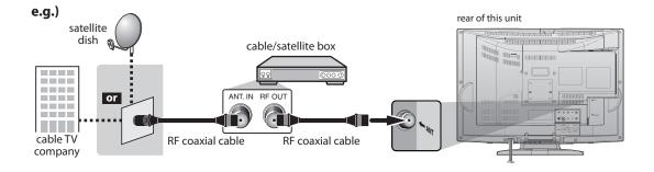
\*Required cables and connecting methods differ depending on the cable/satellite box. For more information, please contact your cable/satellite provider.
